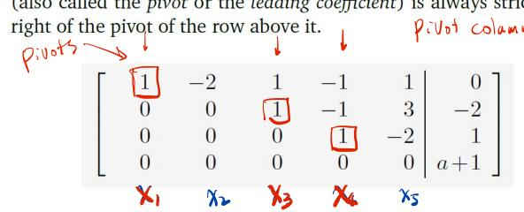
Remark (Basic and Free Variables). The variables corresponding to the pivots in the row-echelon form are called *basic variables* and the other variables are *free variables*. For example, in (2.45),  $x_1, x_3, x_4$  are basic variables, whereas  $x_2, x_5$  are free variables.
