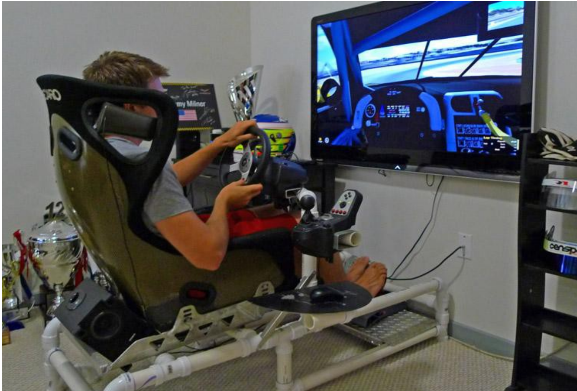
Figure 2. A lower fidelity, do-it-yourself sim racing rig for home usage (courtesy T. Milner).
