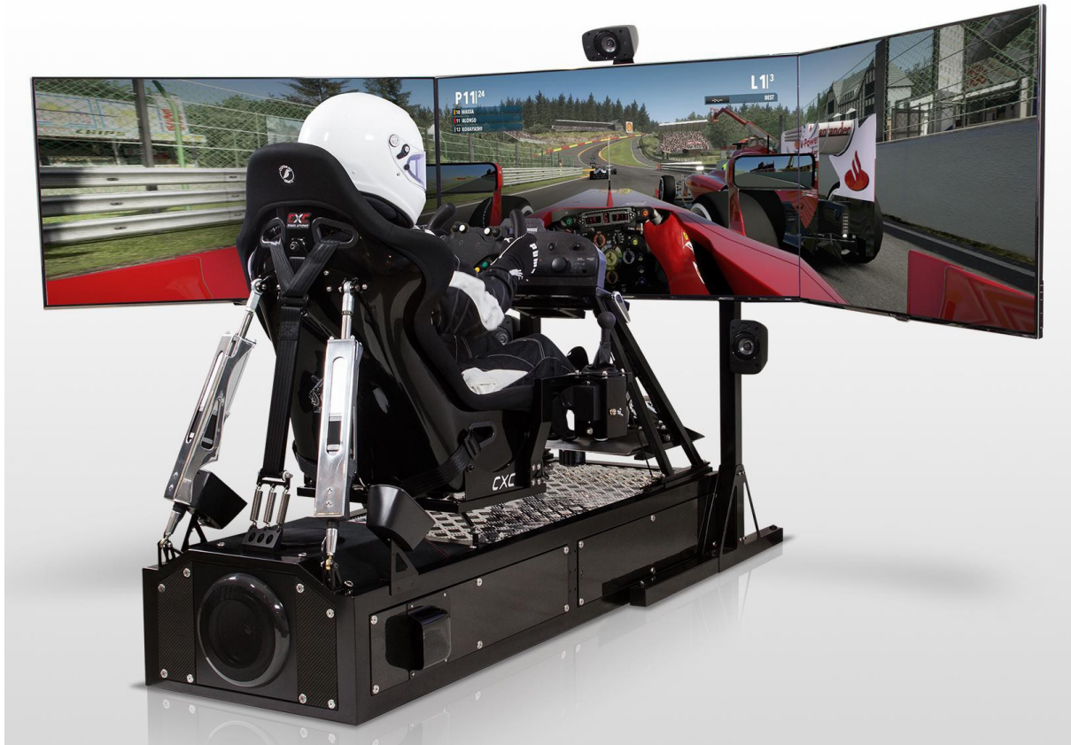
Figure 3. A high fidelity, motion-controlled, multi-display sim racing system suitable for professional, commercial, or in-home usage (courtesy CXC Simulations).
