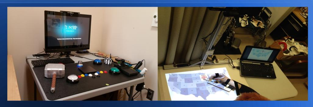
*UI devices*: Game console buttons (large, small), continuous dial, Myo armband, touchpad, joystick, WiiMote, PS Eye, finger pressure force sensor.
