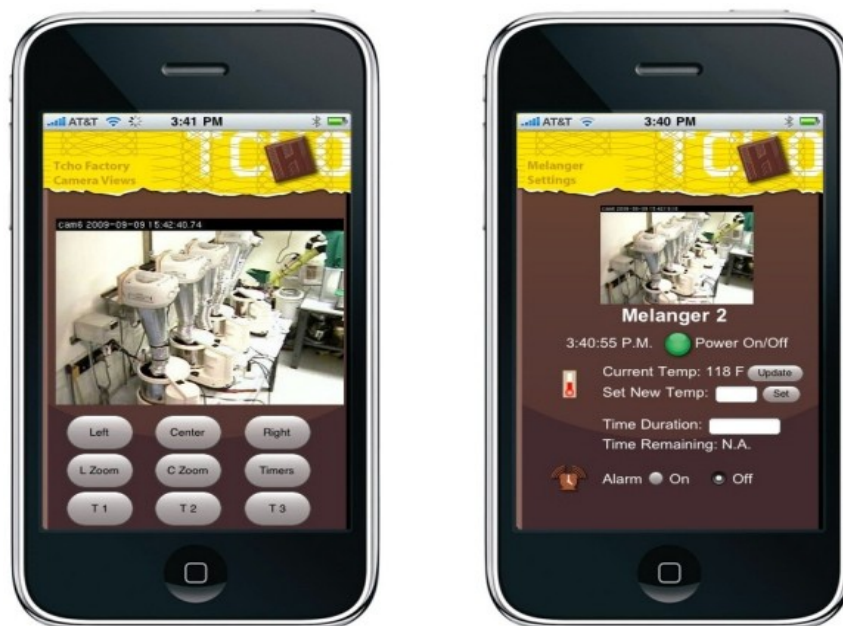
Smart-phone (iPhone) based views for monitoring and controlling devices in the physical TCHO factory, from Back, Kimber, et al. [2010].
