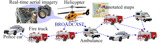
Fig. 1. Dissemination of Mission-Critical Rich Content: An Example Scenario (receivers are from different organizations). Hence, achieving reliability often involves sacrificing transmission/time efficiency, or even making the heavy assumption that no receiver crashes or leaves the network during the dissemination.
