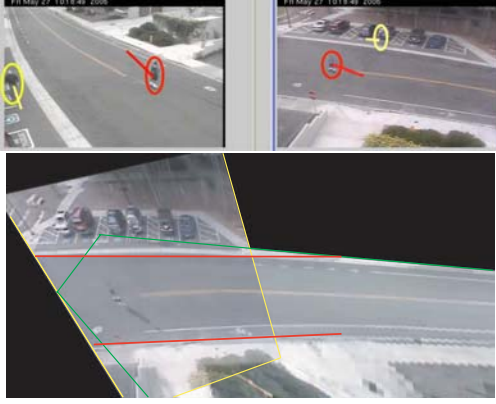
Figure 3. Example of homography mapping. Two perspective views are registered in a common virtual top-down view.
