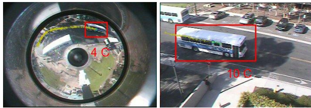
Figure 8: Camera handover between an omnidirectional and a rectilinear camera. The numbers are track IDs in a single camera and letters are IDs assigned across cameras. A bus tracked in the omni camera is identified in the rectilinear camera by assigning the same letter (C).
