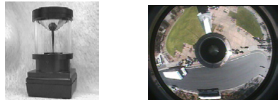
Figure 1. An omni-directional vision sensor (ODVS) and the camera image.
