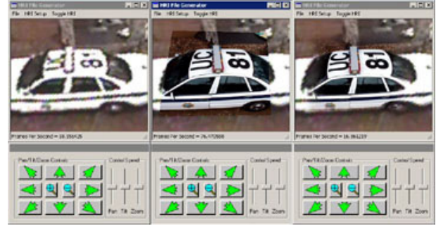
Figure 11: Results of seamlessly integrating a high resolution image to an omni-image. The GUI allows an observer to explore remote sites.
