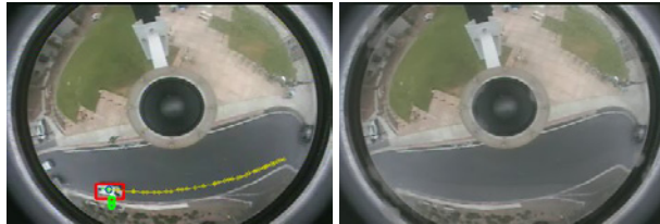
Figure 7: Tracking of a vehicle in omni video sequence. Bounding box is shown in red, with track id in green, and the track history as a yellow line. Image on right shows the current estimate of the background image. Note that the moving vehicle has got removed in the background image.
