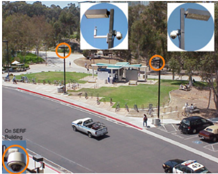
Figure 10. UCSD base node capable of acquiring 16 video streams over a 1 Gigabit fiber optic link.
