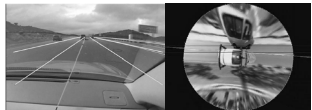
Figure 8 Lane detection using the LISA-Q test bed for both rectilinear (Left) and omnidirectional (Right) vision sensors.
