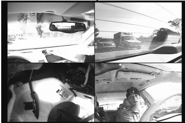
Figure 5 Top left: head cam capture; Top right: rear cam capture; Bottom left: Foot cam (note floating foot over brake pedal); Bottom right: Face Cam
