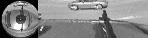
Figure 9 Object detection using an omnidirectional vision sensor (Left - Raw image corresponding to processed image, Right - arrows facing in direction of motion relative to camera.)
