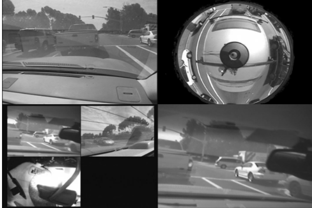
Figure 6 Video data taken from the Q45 Test Bed. (Upper Left – Front View, Upper Right, Omnidirectional Vision Sensor, Lower Left – Rear View/Subject Camera/Near-IR Foot Camera, Lower Right – Subject Camera.)
