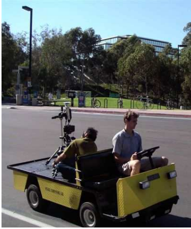
Figure 7: An ODVS camera mounted on an electric cart for a mobile sentry experimental run.
