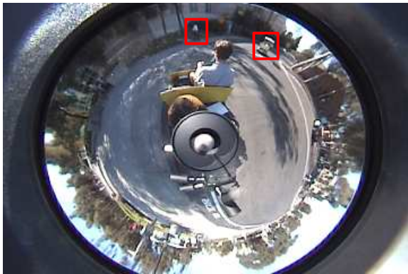
Figure 11: Original image corresponding to a missed events. The moving person and vehicle were far from the camera and near the boundary of region of interest. Also, the camera vehicle was taking a turn, inducing considerable rotational ego-motion in the image.
