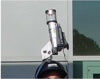
Figure 16: ODVS camera mounted on a helmet. This configuration enables acquisition of snapshots of surrounding people including their faces. However, there is considerable camera rotation due to movement of head and body which should be compensated.
