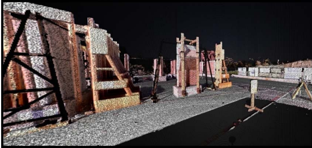
Figure - (A) LIDAR point clouds of structural specimens on the UCSD Outdoor Shake Table (B) with photodraped surface mesh
