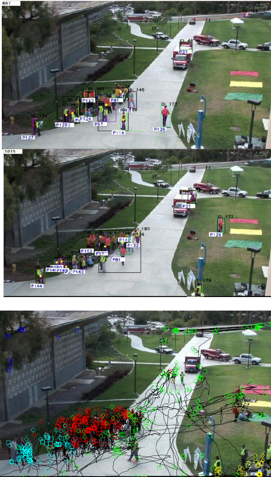
Figure 5. Tracks of people and vehicles observed over a long period in HD Video camera. The personnel can be distinguished from the color of the uniforms. The track start and end points are clustered into 5 clusters using Gaussian Mixture Model.
