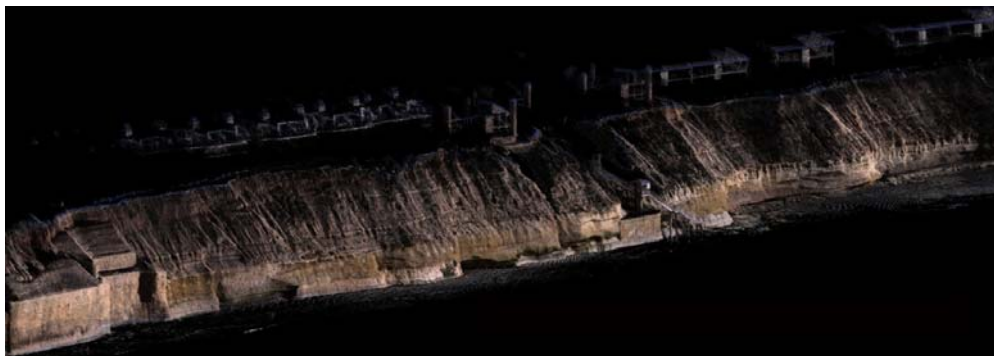
Figure 5 : Georeferenced point cloud dataset of seacliffs at Solana Beach.
