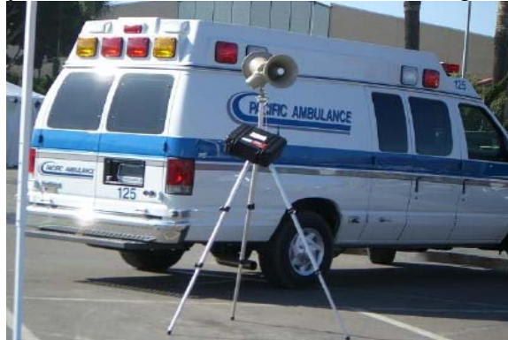
Deployed WiFi “Bullhorn” unit
