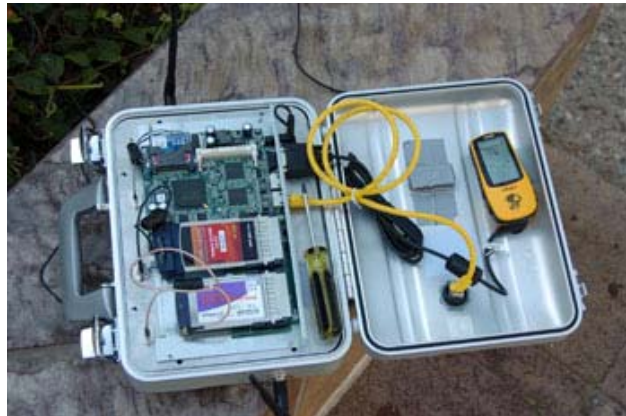
The inside of a CalMesh node
