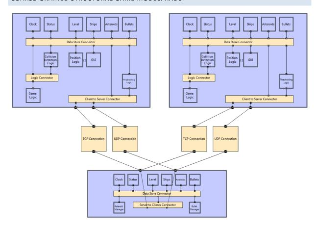
The game is divided into a client and a server application. The above diagram shows two of clients connected to a server, all of them with their internal component structure. The game architecture does not pose any explicit limits on the number of clients simultaneously connected to the game server.
