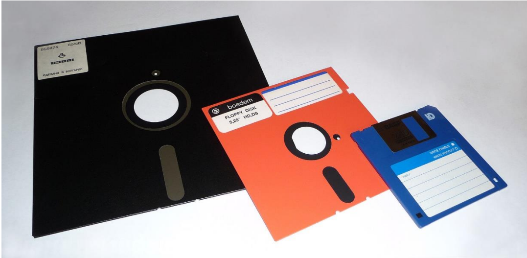
Floppy disk drives 1970's~2000's 100 KiBs to 1.44 MiB
