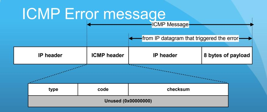
ICMP error messages include the complete IP header and the first 8 bytes of the payload (typically: UDP, TCP)
