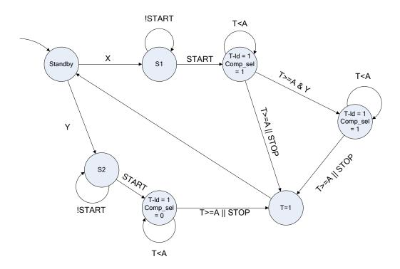
In fact there is a timing issue in each of the states that increments T. To solve the timing issue we have to add a "dummy" state for each problematic state. This "dummy" state is just supposed to provide one more clock cycle for the register to load the value. All the incoming edges still enter to the original state. On the other hand all the outgoing edges exit the "dummy" state.
