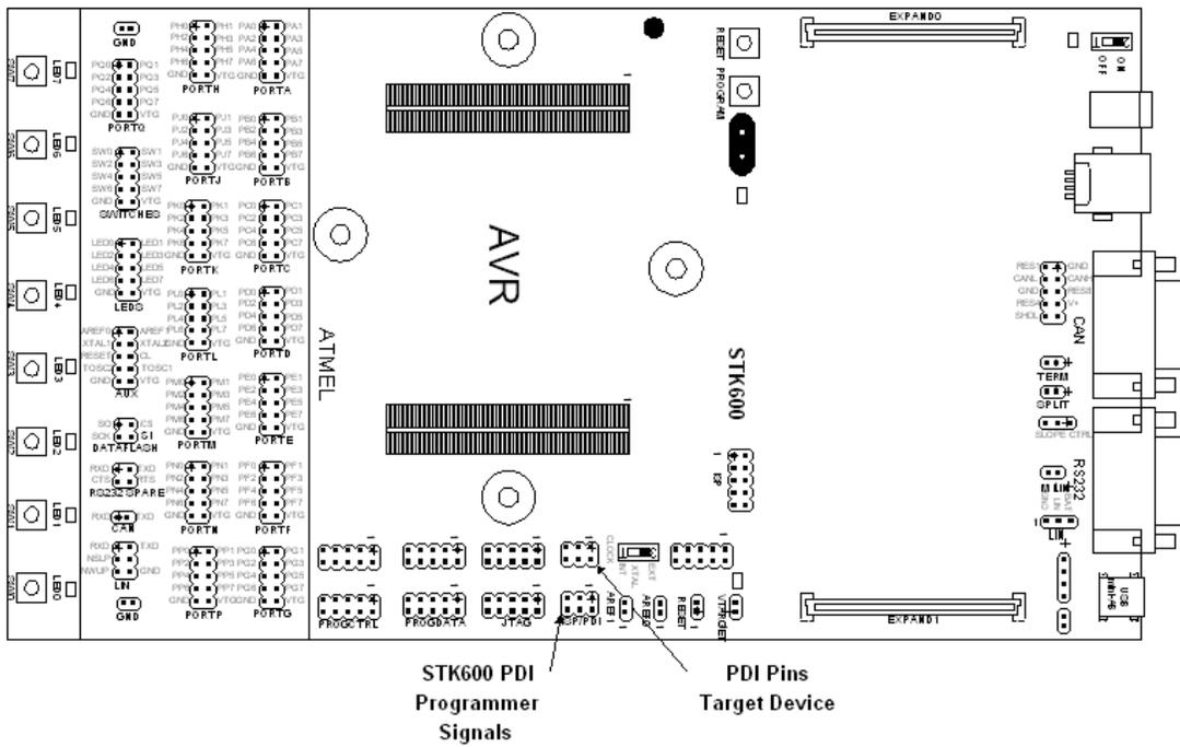
The PDI interface requires two of the device's pins, PDI\_DATA and PDI\_CLOCK. On STK600, they are found on the ISP/PDI connector.
