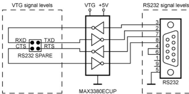
If the RTS and CTS lines are not controlled by the AVR, a jumper shorting the RTS and CTS pins on the "RS232 SPARE" header can resolve communication problems, if the PC side expects these handshake lines to be active.
