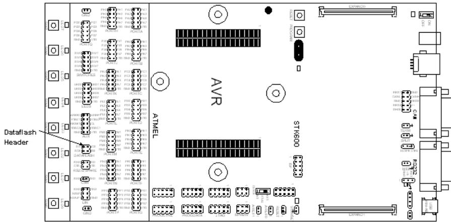
The dataflash can be connected to the I/O pins of the microcontroller sockets. The 4-pin header marked "DATAFLASH" can be used for connecting the SPI interface of the dataflash to the I/O pins on the target AVR microcontroller in the socket. 2-wire cables are included with STK600 for connecting the dataflash to the I/O pins. The connection of the I/O pins is shown on the picture below.
