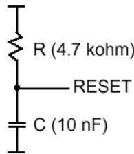
If the external pull-up resistor is too strong (i.e  $\ll 4.7\text{k}\Omega$ ), STK600 may not be able to pull the RESET line low.
