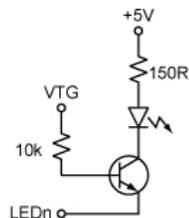
To light one of the LEDs, the corresponding pin found on the LEDs header must be pulled to GND.
