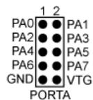
The other port connectors are identical, only with different signal names.
