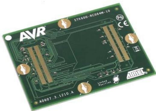
A set of spring loaded connectors make the connection between the motherboard, routing card and socket card. Clips or screws hold the stack of cards together.
