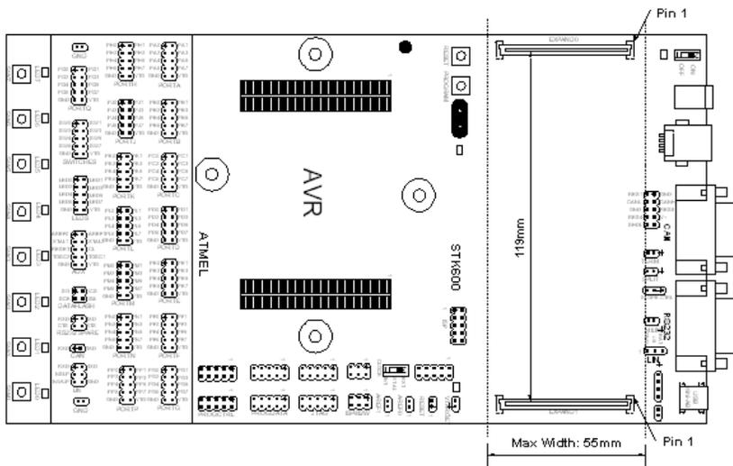
The connectors to be used on an expansion board is manufactured by FCI and has P/N: 61082-101402LF. See also [www.fciconnect.com](http://www.fciconnect.com) for more information.
