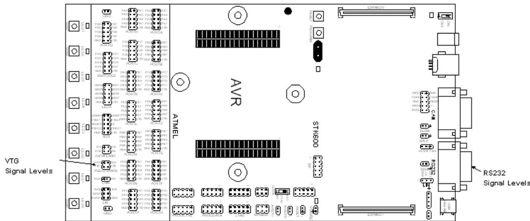
To use the RS232 interface, the AVR's UART pins must be connected to the appropriate pins on the "RS232 SPARE" pin header. Use a 2-wire cable to connect the AVR's RXD and TXD pins to the pin header. The "RS232 SPARE" pin header is found in the target header section, while the DSUB marked "RS232" is located on the other end of the card.
