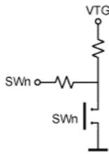
When pressing one of the switches, the corresponding SW pin on the SWITCHES header will be pulled low. When the switch is released, the switch's 10k pull-up will pull the line to VTG. The 150 Ohm resistor prevents a large current to flow to ground in case of wrong wiring.
