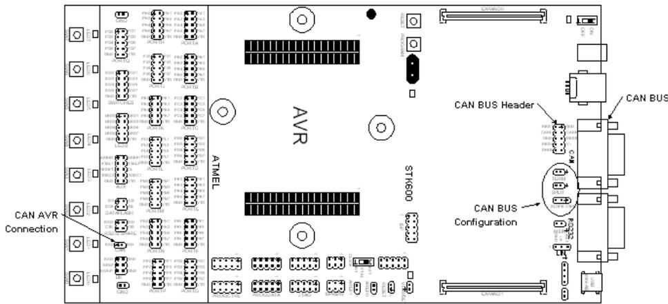
If a network termination is needed (CAN baudrate higher than 100 Kb/s), the 'TERM' jumper can be mounted to insert a 120 ohms resistor between CAN-H and CAN-L.
