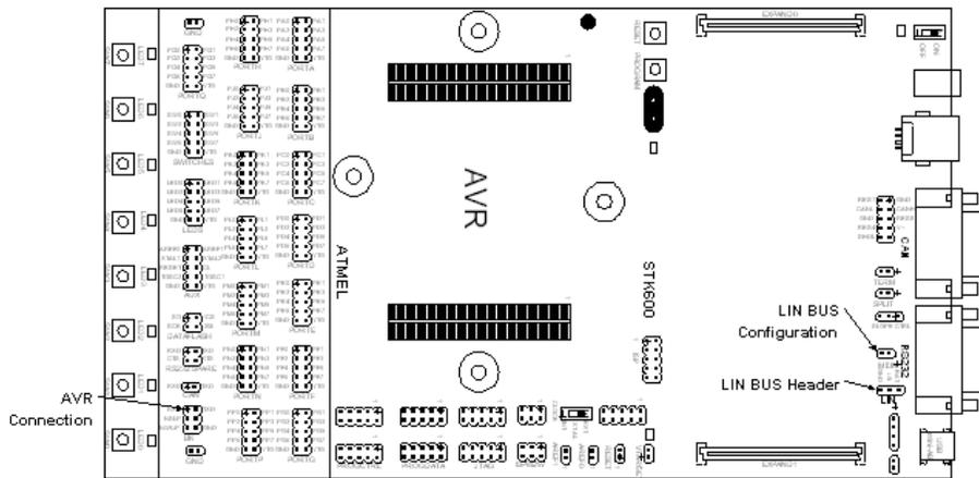
The 'M LIN' jumper provides the master node pull-up, required if the application running on STK600 is the LIN bus master.
