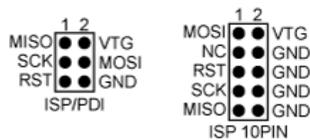
It is not necessary to remove the ISP cable while running a program in the AVR. The port pins used for ISP programming can be used for other purposes in your program.
