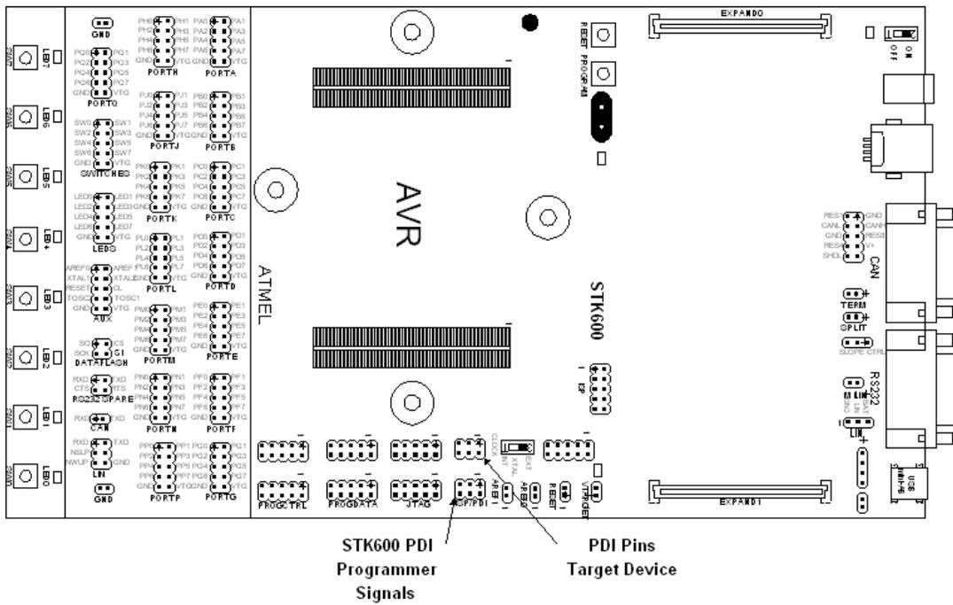
The TPI interface requires two of the device's pins, TPIDATA and TPICLK, in addition to the RESET pin. On STK600, they are found on the ISP/PDI connector. Note: TPI is only supported on-board, i.e it is not possible to program a device on an external board through the TPI interface.
