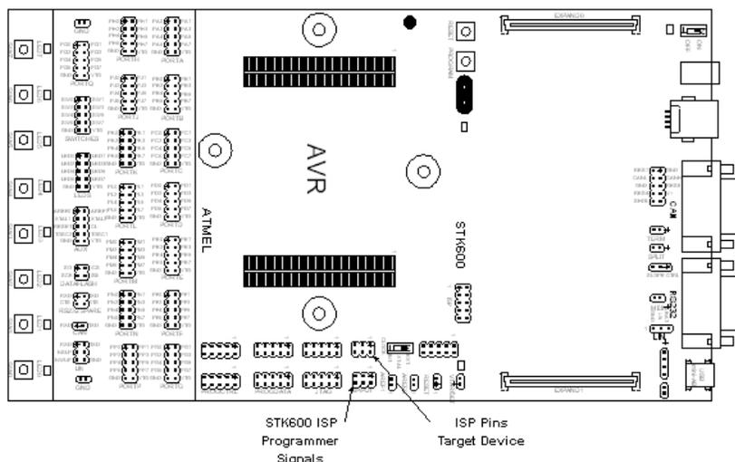
Note that the ISP frequency (SCK) must be less than 1/4 of the target clock. The ISP frequency is set by the STK600 programming dialog in AVR Studio.
