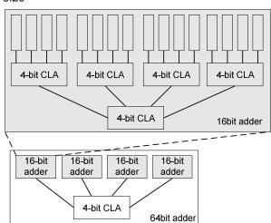
delay of 64-bit hierarchical carry-lookahead adder : 4\*2=8, gate delay delay of 64-bit carry-ripple adder : 64\*2=128, 128 gate delay
