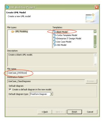
h) Select Main under UseCase\_DVDStore in the Model Explorer. Expand the "Use Case Diagram" section in the Palette. Select the objects you need to create for the next step using the Use Case Diagram Palette.
