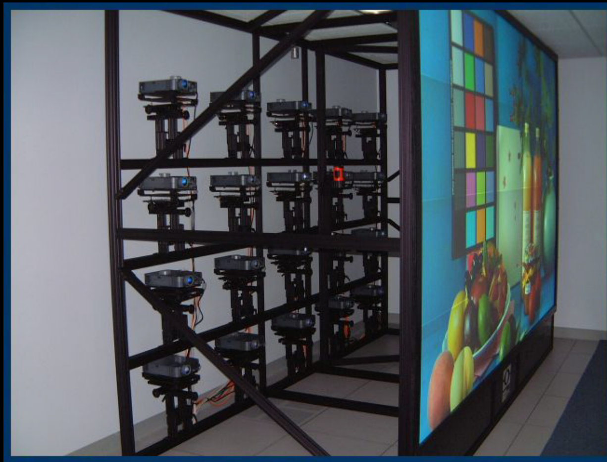
Commercially available 20-projector system from Visbox, Inc.
