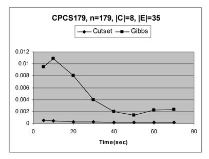
MSE vs. #samples (left) and time (right) Non-Ergodic (1 deterministic CPT entry) |X| = 179, |C| = 8,  $2 <= D(X_i) <= 4$ , |E| = 35
