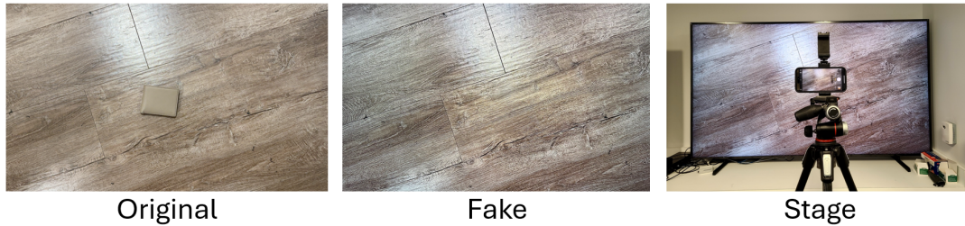
Figure 2: An example of a recapture attack on a provenance-based secure camera.
