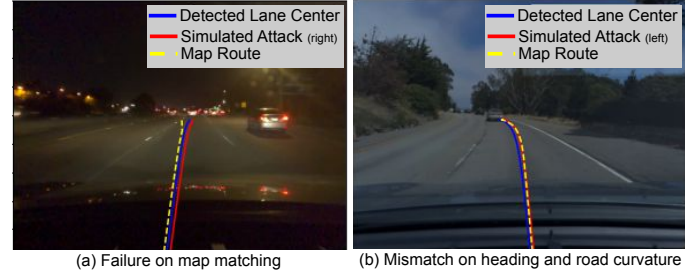
Fig. 4: Case studies on false positives: (a) The map is associated with the wrong point as the road curve should start at a further point; (b) the vehicle heading does not match with the road curvature while the detected lane center looks accurate.
