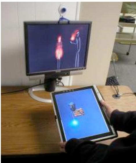
Figure 1: Embodied Mobile Agents may animate seamlessly between a desktop computer and a tablet PC.
