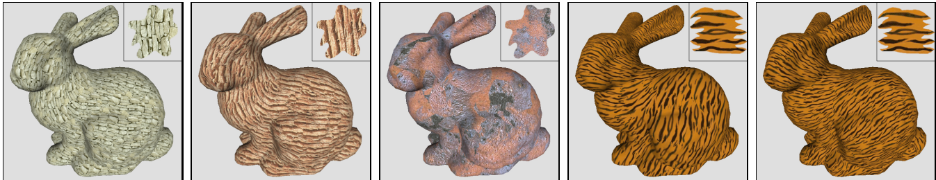
Figure 1: Four different textures pasted on the bunny model. The last picture illustrates changing local orientation and scale on the body.
